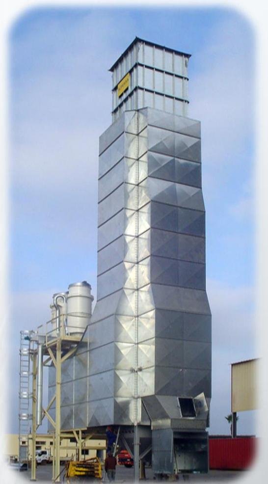
Aeration system with efficient dust control. Ciclofans CF-30, motor 22 kW, complete, vertical position, with miniciclone, air return hose, with recovery of the dust, efficiency 94%. Unitary flow: 27.160 m<sup>3</sup>/h.
